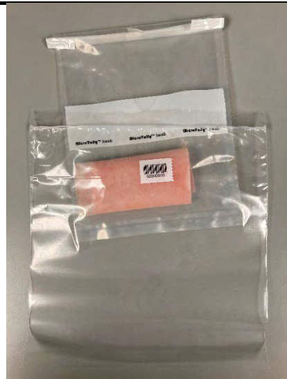
Fig. 10: Insert bagged cloth into a zipper lock bag for shipping
